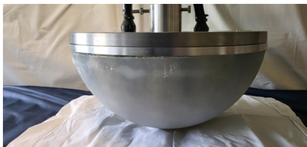
Figure 3a: Hemispherical Indenter used for test SS-1:2019 Section 6. Not actual test rig used – image for illustration purposes only.
